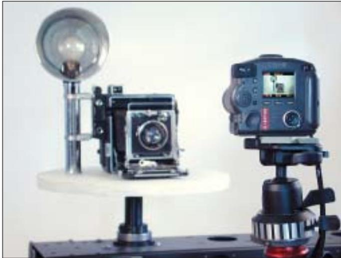
Figure 9.6: A simple object movie shooting setup: the object is mounted on a turntable, and the camera is on a tripod. (Photo by Scott Highton)
